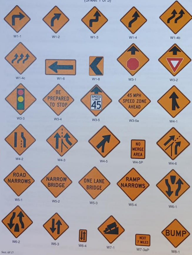
Figure 6F-4. Warning Signs and Plaques in Temporary Traffic Control Zones (Sheet 1 of 3)
