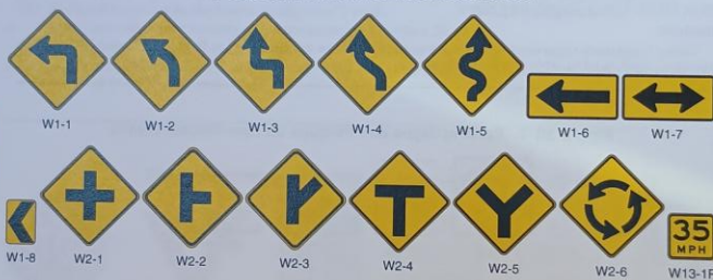
Figure 5C-1. Horizontal Alignment and Intersection Warning Signs and Plaques and Object Markers on Low-Volume Roads
